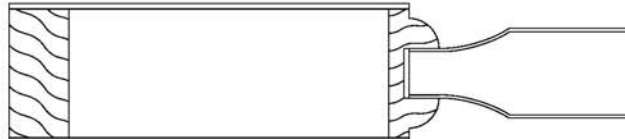
Membrane pressed veneer raised panel Premium or Custom grades (scoop panel raise) Premium grade must be at the request of the architect or specifier
