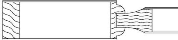
Rim banded veneer raised panel Premium or Custom grades (scoop panel raise)
